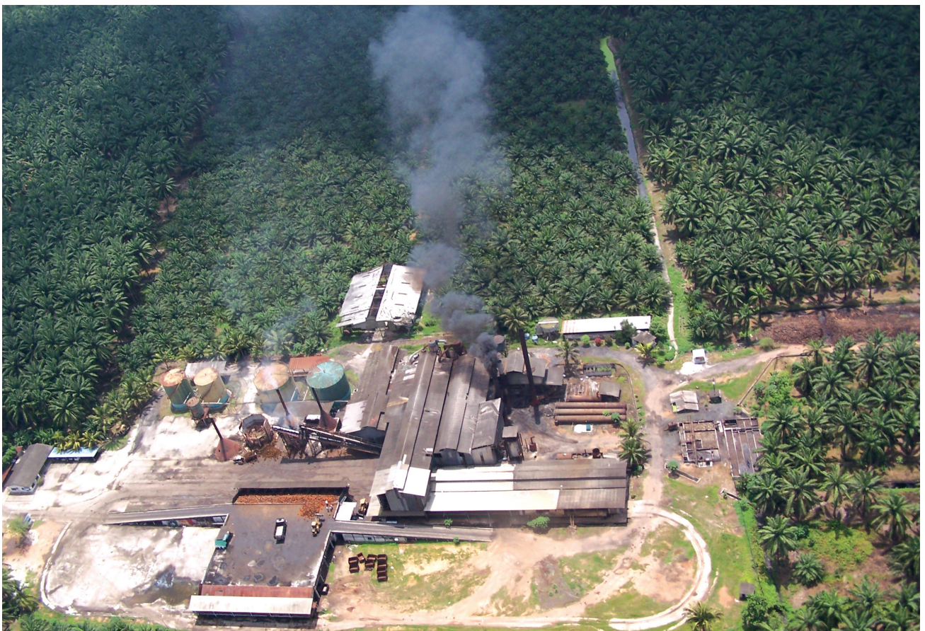
Black smoke emissions : Facility without air pollution control equipment (DOE Photo Library)
