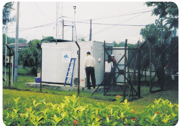
Gambarfoto 5.2 JAS: Stesen Pemantauan Kualiti Udara Automatik Photo 5.2 DOE : Automatic Air Quality Monitoring Station
