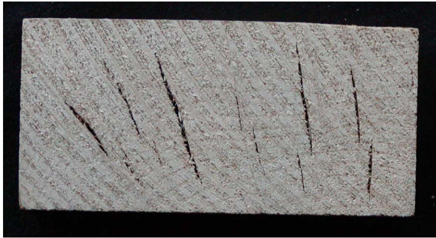
Figure 4 Honeycomb can occur if the internal tensile stress is high enough. This occurs when the core of the piece is near or below the fiber saturation point. These cracks would not be visible on the end of the piece.
