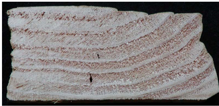
Figure 2 Capillary forces, especially in low density species with high moisture content, can result in collapse. Wood can be steamed to recover minor collapse if no cracks have occurred.
