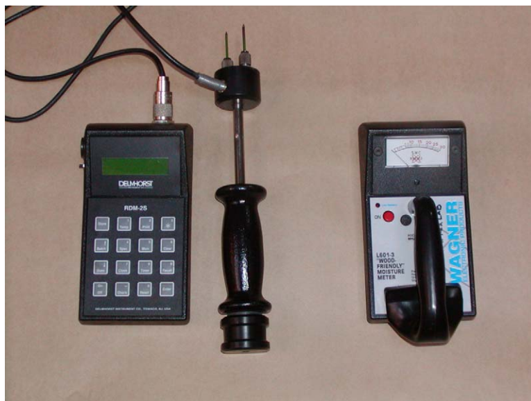
Figure 9 Pin-type (left) and capacitance-type (right) hand-held moisture meters.
