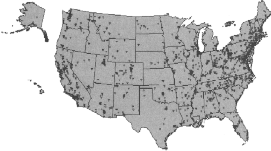
Fig. 8.12. The SLAMS consist of a network of ~4000 monitoring stations whose size and distribution is largely determined by the needs of State and local air pollution control agencies to meet their respective State Implementation Plan (SIP) requirements. Source: US Environmental Protection Agency 2006, The Ambient Air Monitoring Program , http://epa.gov/oar/oaqps/qa/monprog.html#SLAMS ; accessed on October 30, 2006.
