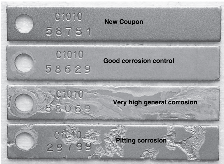
Figure 5.12 Corrosion coupons illustrating the types of corrosion
