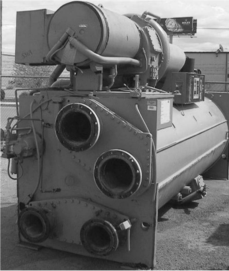
Figure 6.2 A photo of a centrifugal compressor and chiller
