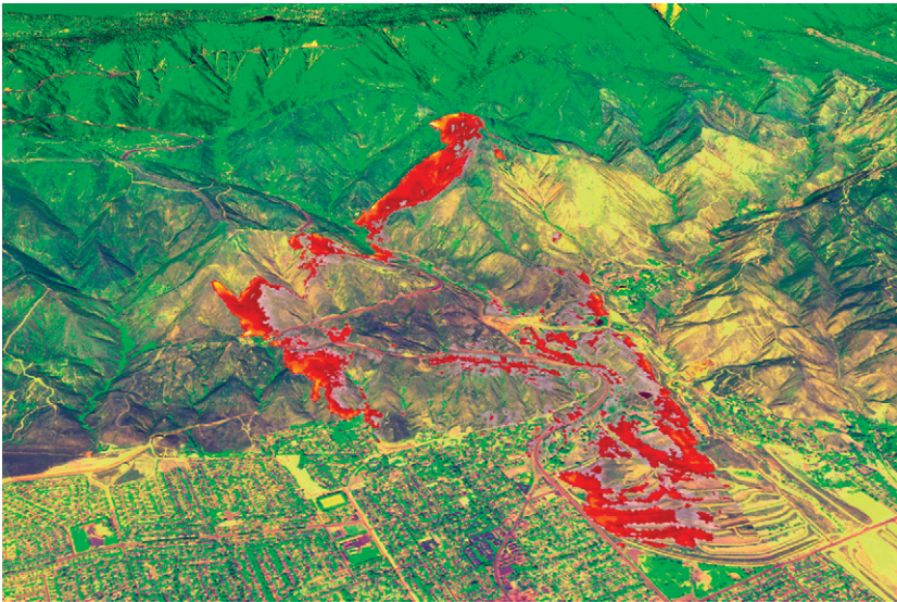
Figure 6.10a. Old Fire, San Bernardino County, CA, as viewed from the southwest at 11:14 Pacific Daylight Time, October 25, 2003, by the PSW FireMapper thermal-imaging radiometer. Color-coded surface temperatures, which reflect fire intensity, are presented as measured in the thermal infrared and posted as an off-nadir overlay on a prefire, multispectral image (with red, near-infrared, and thermal-infrared light shown in red, green, and blue) at http://www.fireimaging.com . Here, a moderate Santa Ana wind is driving the fire to the south and southeast through chaparral and light fuels on hillsides into urban vegetation and structures in the City of San Bernardino. Note the lack of fire activity where the Old Fire encountered the perimeter of the June 1–7, 2002, Arrowhead Fire (yellow vegetation at right of center). Fire at the lower right is burning on a spreading ground, which is used to recharge groundwater. At the time of this image there was little fire activity in the urban area below the burned foothills at lower center.
