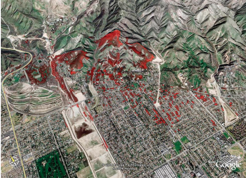
Figure 6.10b. Old Fire, Del Rosa neighborhood, City of San Bernardino, as viewed from the southwest at 13:56 PDT, October 25, 2003, by the PSW FireMapper. Color-coded surface temperatures are presented as an off-nadir overlay in Google Earth as shown as a standard product in near real time at http://www.fireimaging.com/ . Here the fire has progressed into the urban area partly by wind-blown fire brands, a large portion of which apparently originated from eucalypts, palms, or other urban vegetation. A long fire incursion is visible along a flood-control facility at lower left-center. Fire-involved structures are readily identified in this image; rapid communication of such imagery could aid firefighters in showing the extent of the fire's incursion into the city and the location of newly involved structures.
