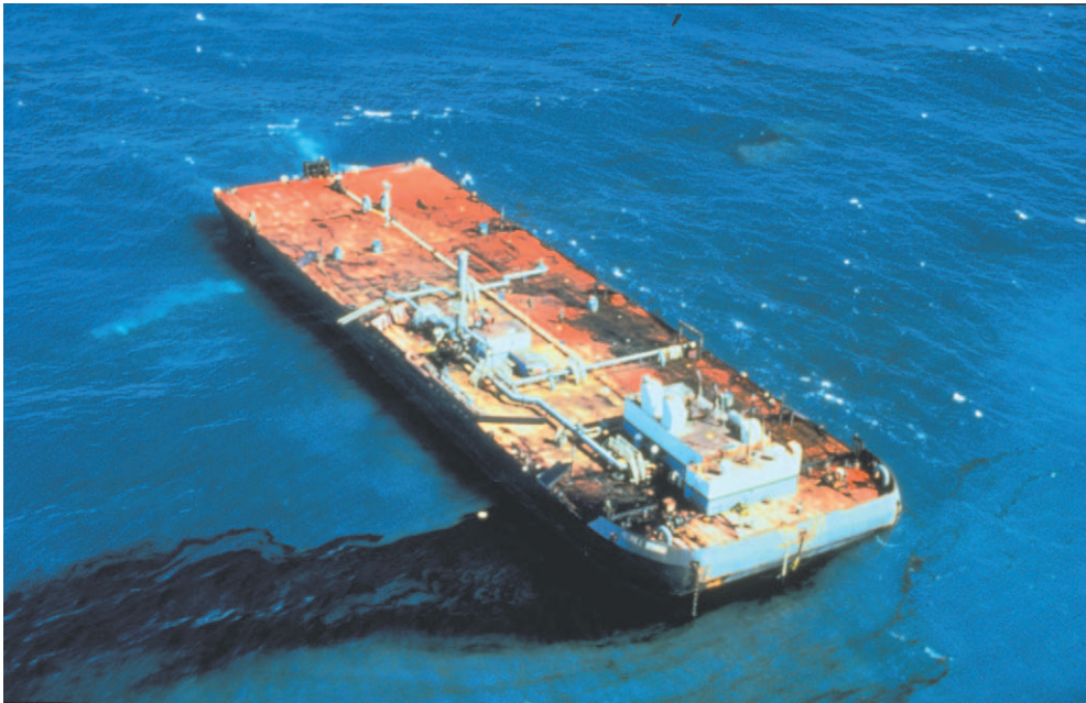
The Morris J. Berman tank barge on a two-day voyage to St. John, Antigua, pulled by the tugboat Emily S. broke an improperly repaired towline and ran aground on a reef off San Juan, Puerto Rico, spilling 798,000 gallons of No. 6 diesel fuel. See Ornitz (1996) for a review of this spill. Photograph courtesy of NOAA Office of Response and Restoration.
