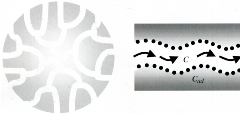
Figure V.2.6. Diffusion of soluble and adsorbed pollutant Left: porous particle. Right: pore in porous particle.
