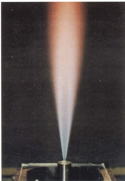
CHAPTER 2, FIGURE 4 A hydrogen-air jet diffusion flame established on a 1.43-mm-diameter stainless-steel burner nozzle (hydrogen flow rate at the burner port is 500 m/s) (Takahashi et al. , 1996).
