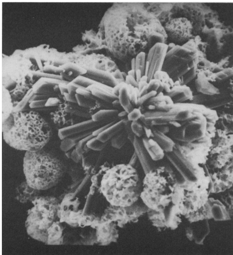
Fig. 2. Carbonaceous particles emitted by combustion processes enucleating gypsum crystals under laboratory controlled conditions (wetting in absence of sulphur dioxide) (scanning electron micrograph, 2500x).
