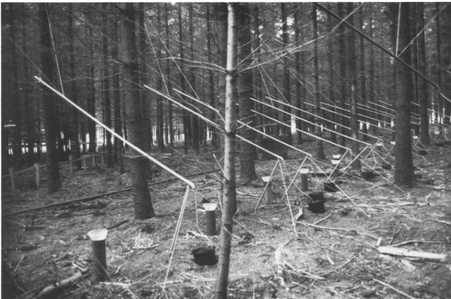
FIGURE 3.5 ( continued ) Illustration of instrumentation used for flux gradient measurements at the Elspeetsche Veld and throughfall measurements at the Speulder forest.
