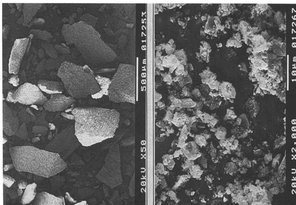
Figure 5 SEM of ceramic waste CSP before grinding, 50x. Figure 6 SEM of ceramic waste CSP-4 after grinding, 2000x.
