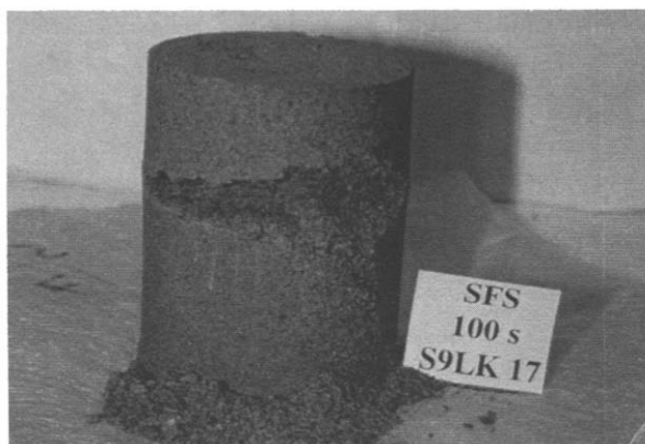
Fig 3. A sample after the SFS freeze-thaw test.
