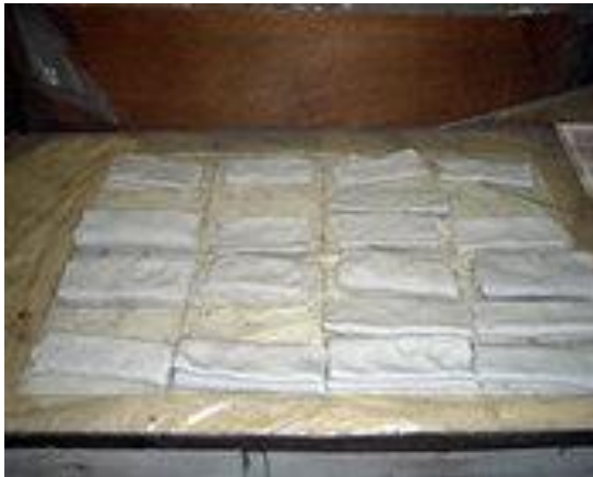
Pulp after dewatering
