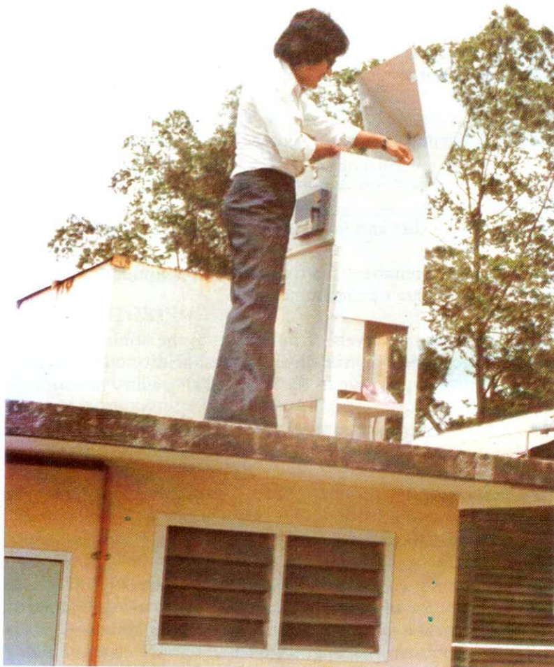
AIR QUALITY MONITORING EQUIPMENT IN OPERATION: High Volume Sampler for particulate measurement.
