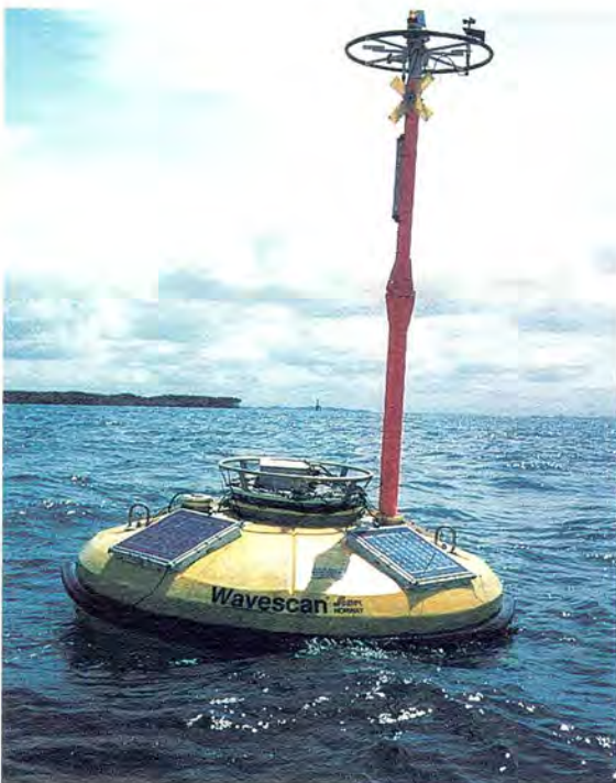
Wavescan Buoy and Telemetry System at Tanjung Piai, Johor
