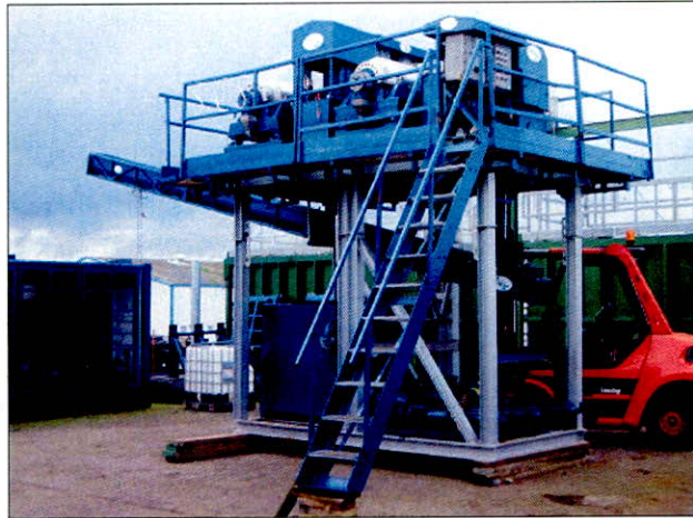
Twin decanter centrifuge system for refinery wastewater clarification and dewatering
