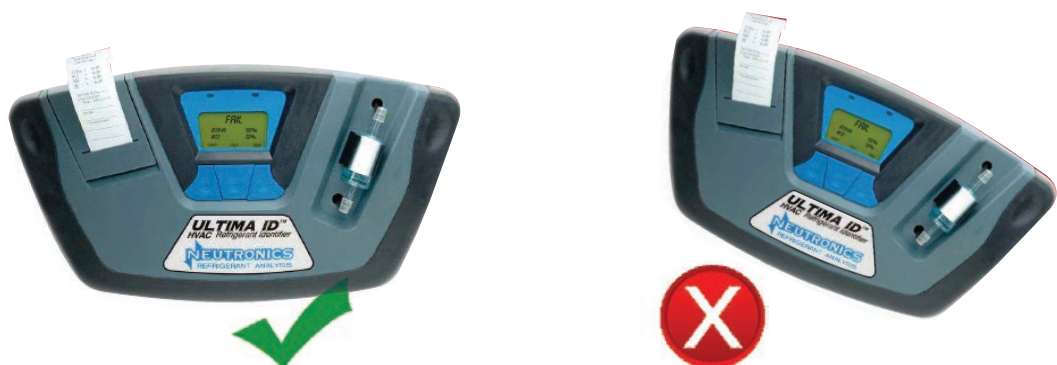
Figure 10.10: Place the Identifier on a flat and sturdy surface
