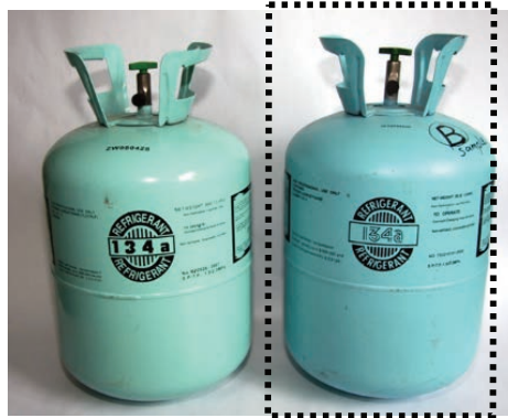
Figure 10.1: Example of counterfeit Refrigerant (sample on right)
