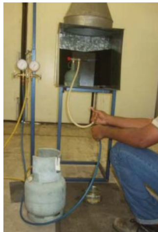
Figure 10.5: Halide flame test
