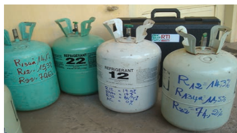
Figure 10.6: Fake refrigerant cylinder
