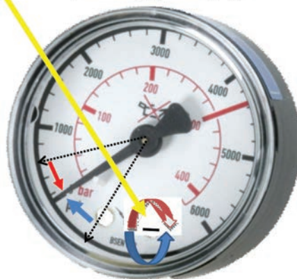
Figure 11.2: Zero error of the gauges
