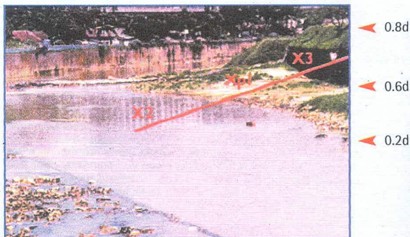
Plate 11: Sampling procedure ( d =depth, x =sampling point)
