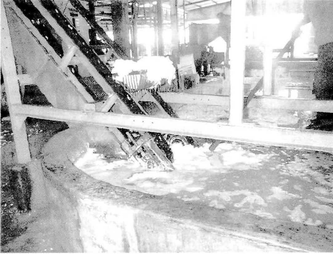
← Sources of effluent: Materials washing
