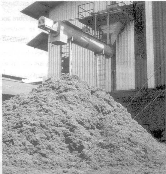
↑ Shell and fibre are used as boiler fuel ↑
