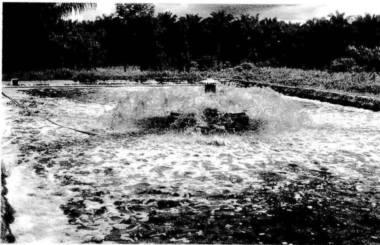
← A Typical Aeration System
