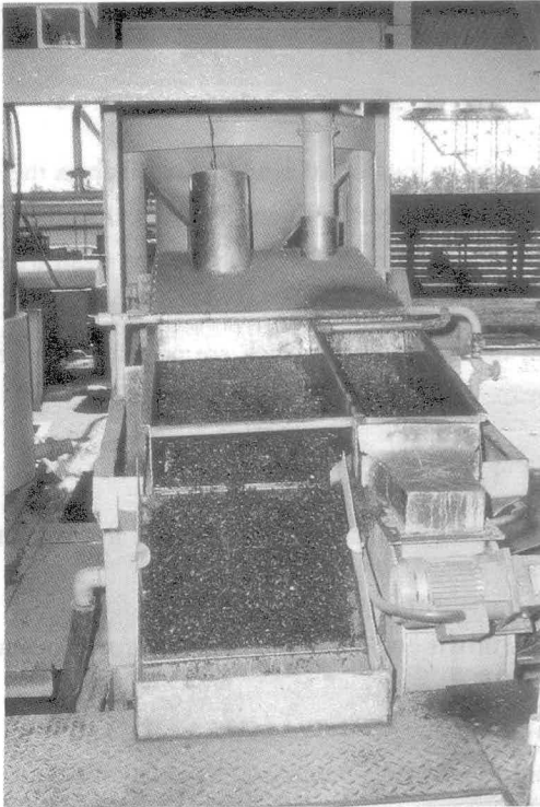
← Hydrocyclone is employed to separate the kernels and shells
