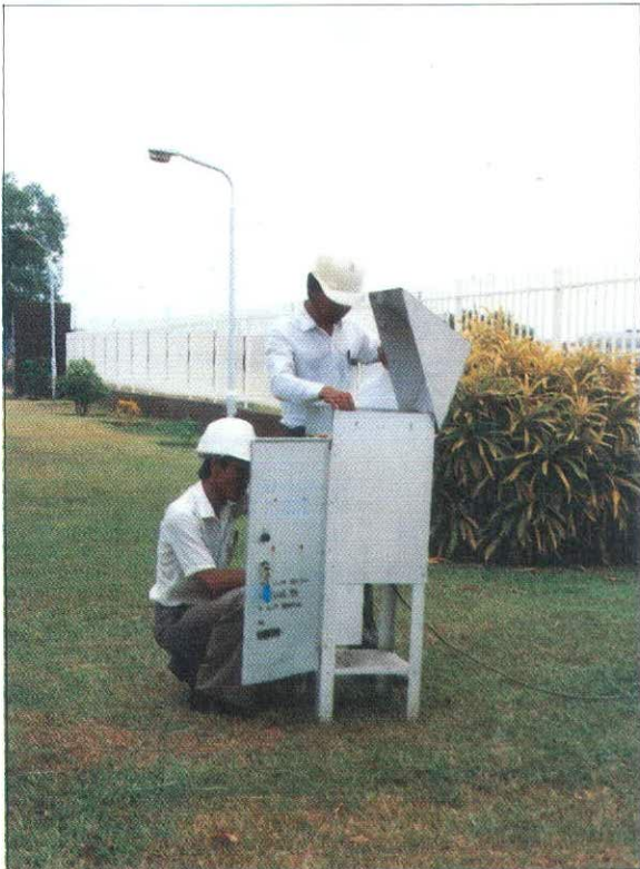
Air Sampling for Suspended Particulate Matters.
