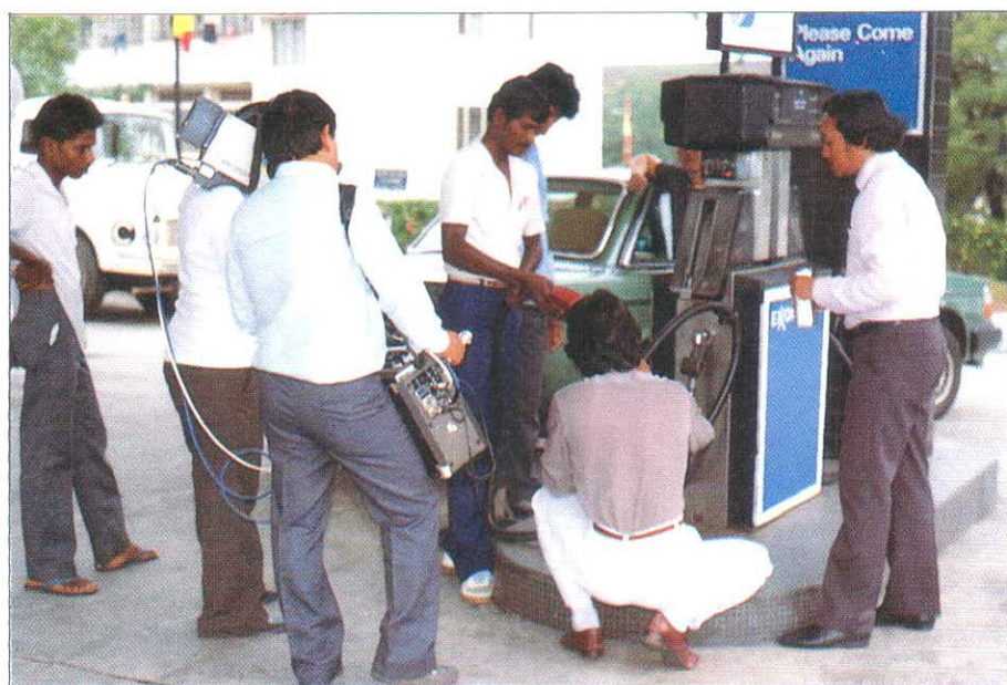
Sampling of Gasoline for Testing of Lead Content.
