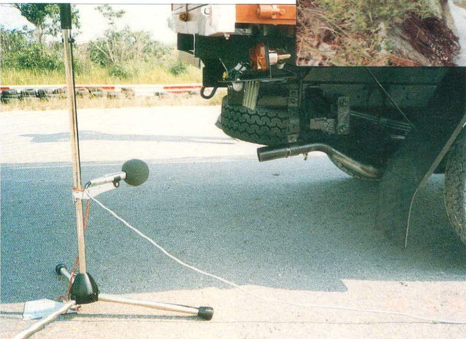
Motor vehicle noise measurement
