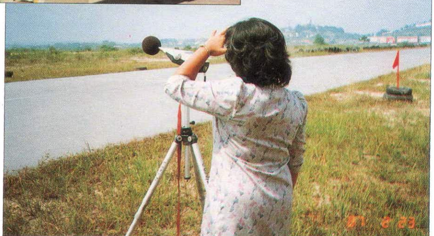
Motor vehicle noise measurement
