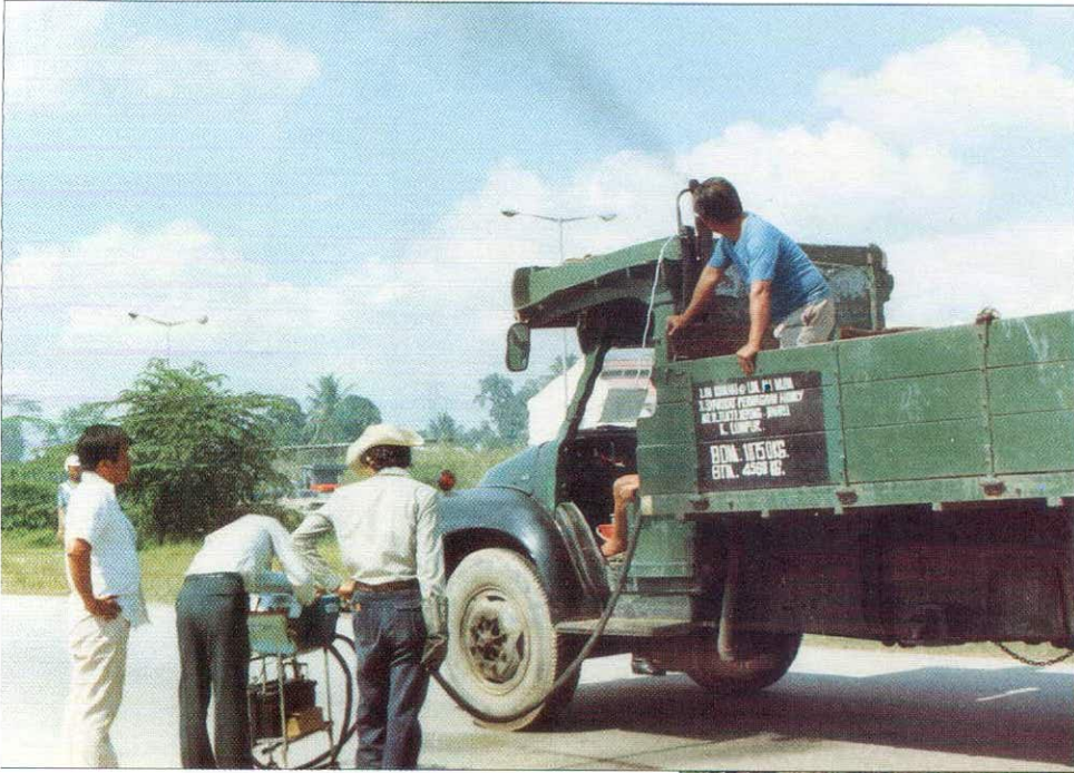
Measurement of dark smoke emission
