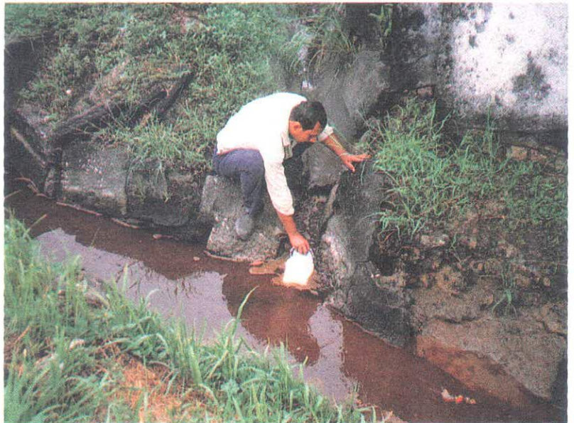
Water Sampling at Final Discharge Point of a Crude Palm Oil Mill during an En- forcement Visit
