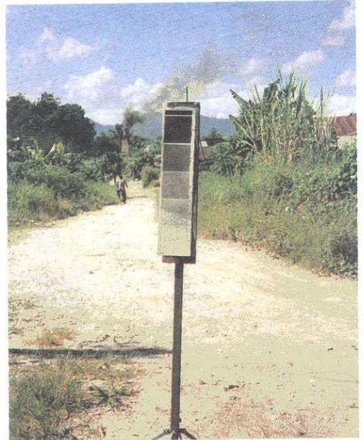
Measurement of Black Smoke Emission Using Ringelmann Chart
