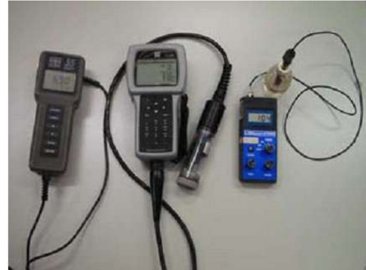
Examples of the various types of field meters available. From left to right: a dissolved oxygen meter, a multi-parameter meter and a redox meter.
