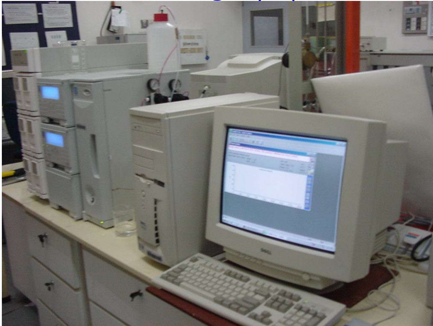
Fig 7: Ion Chromatography -DX 500
