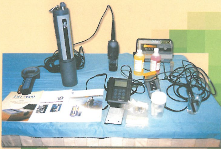
Photo 11 : Multiprobe Sonde for In-situ Water Quality Monitoring (DOE Photo Library)
