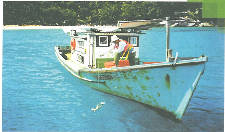
Photo 13 : Marine Water Quality Grab Sampling (Van Dorn Sampler) (DOE Photo Library)
