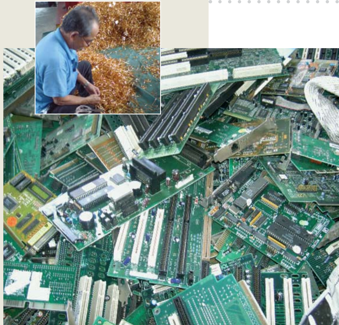
Inset: Manual retrieval of valuable components in e-waste during partial recovery process
