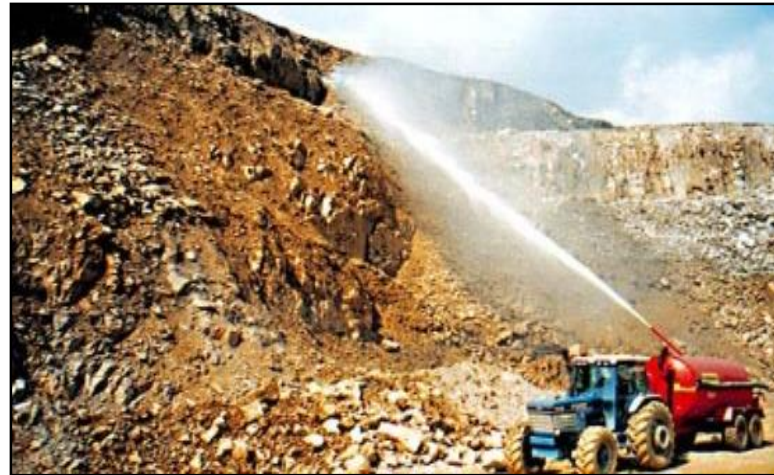
Spraying faces and stockpiles to reduce dust exposure
