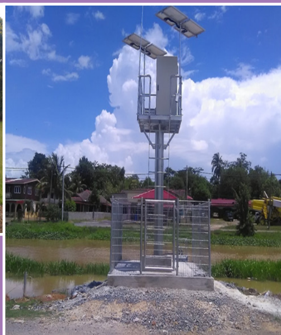
Stesen Pengawasan Kualiti Air Sungai Automatik ◀ The Continuous River Water Quality Monitoring station
