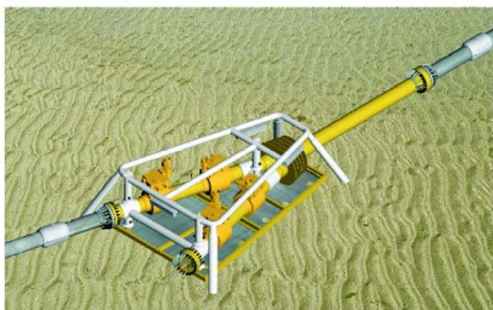
Pipeline End Manifold (PEM)
