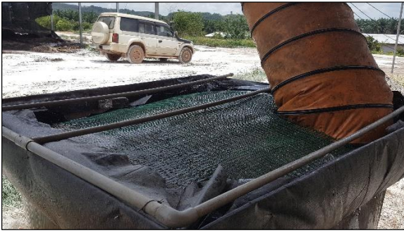
(b) A self-made odour scrubbing and filtering system using a combination of chemicals (e.g. sulfuric acid) and rice husks, for treating odour from the chicken droppings storage. The system was inefficient as the odour actually increased by 25% resulting in an average 4017 OU/m 3 .
