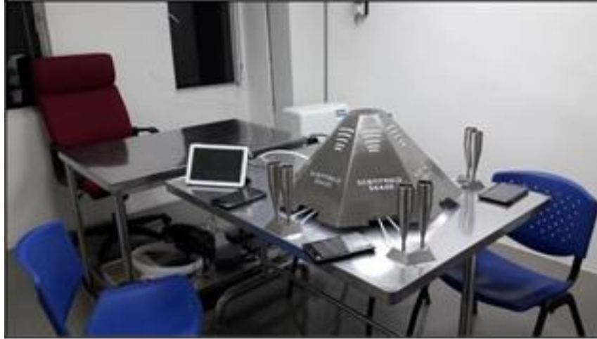
Figure 3.3 Scentroid SS400 dynamic olfactometer for at Universiti Sains Malaysia Odour Laboratory for the determination of odour concentration
