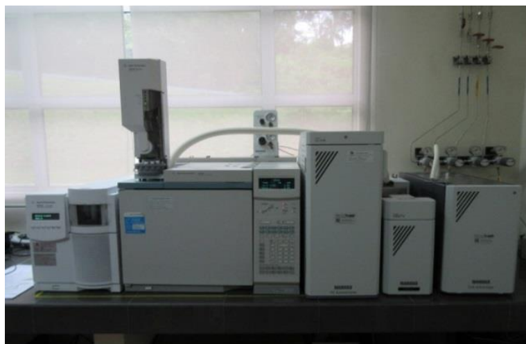
Figure 6 Thermal Desorption (TD) System coupled with Gas Chromatography-Mass Spectrometer (GC-MC) method
