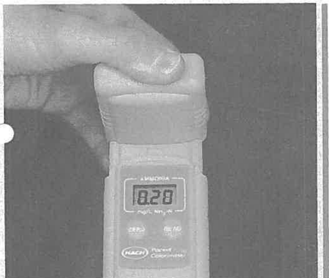
Fig. 17.3: Measuring ammonia using an ammonia analyzer
