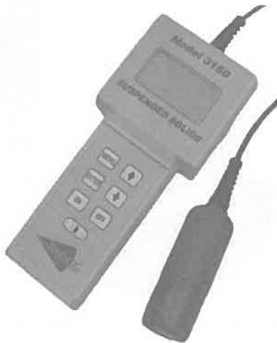
Fig. 17.7: Suspended solids meter
