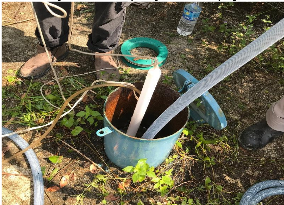
Figure 4-4 Example of groundwater sampling
