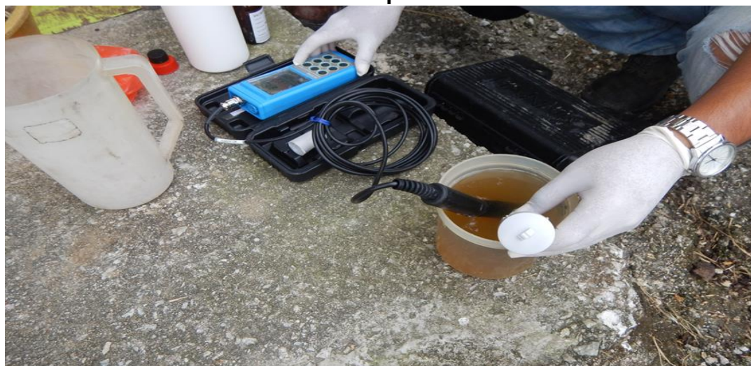
Figure 4-2 Example of water quality testing with a meter on a collected sample
