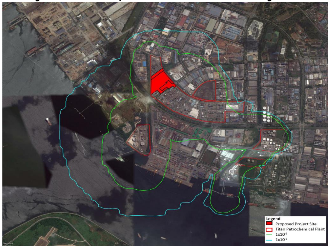
Figure 5-15 Example of Individual Risk Contours using PHAST
