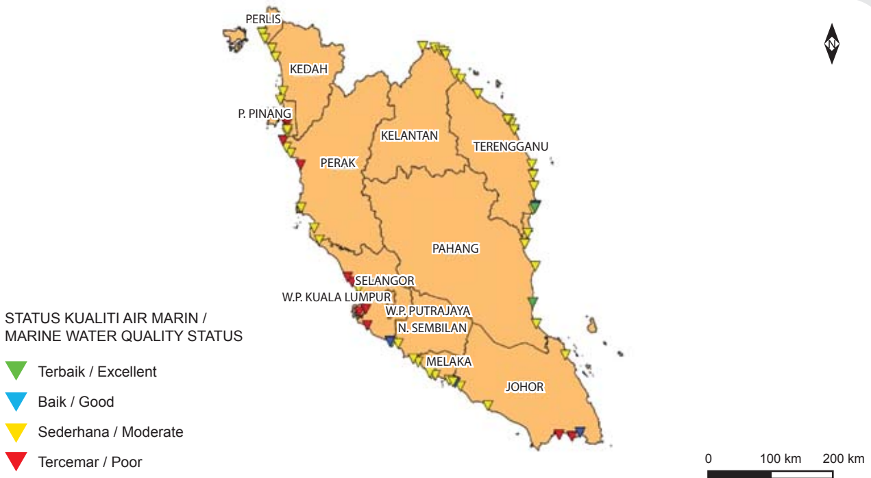
Rajah 4.3 : Status Kualiti Air Marine mengikut Lokasi Stesen Pengawasan bagi Muara Sungai di Semenanjung Malaysia Figure 4.3 : Marine Water Quality Status based on the Location Monitoring Stations for Estuary at Peninsular Malaysia
