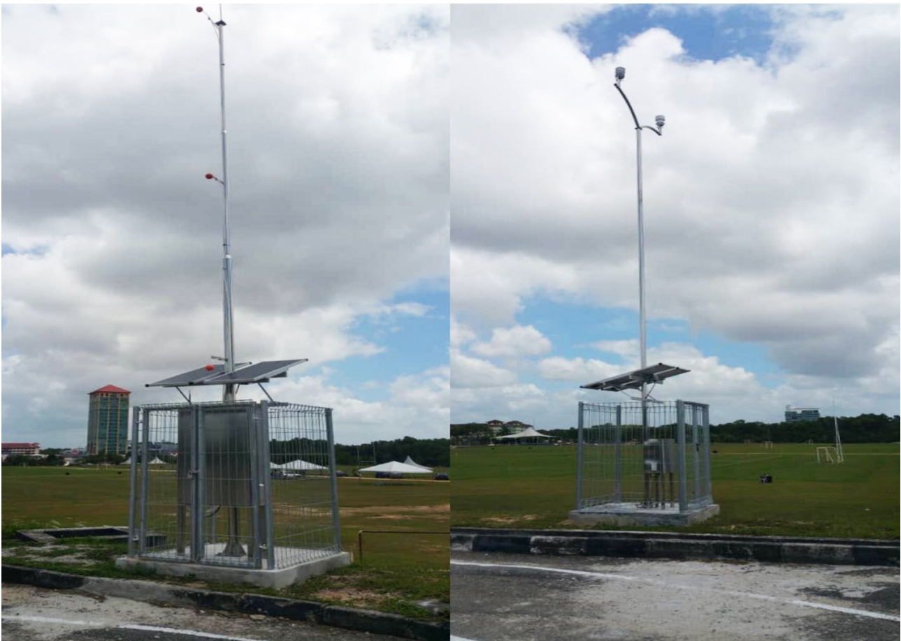
HAP 12, Stesen TVOC (kiri) dan Stesen Meteorologi (kanan) di Pasir Gudang, Johor HAP 12, TVOC Station (left) and Meteorology Station Located in Pasir Gudang, Johor
