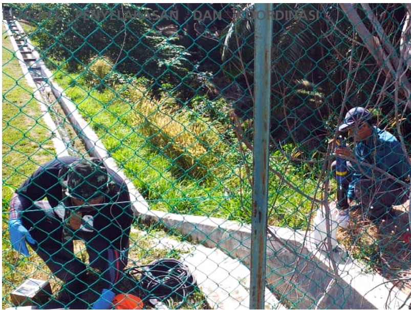
Persampelan In-Situ di Takat Pelepasan Salah Satu Loji Kumbahan yang Diperiksa di Merlimau In-Situ Sampling at the Point of Discharge at One of the Inspected Sewage Plants in Merlimau
