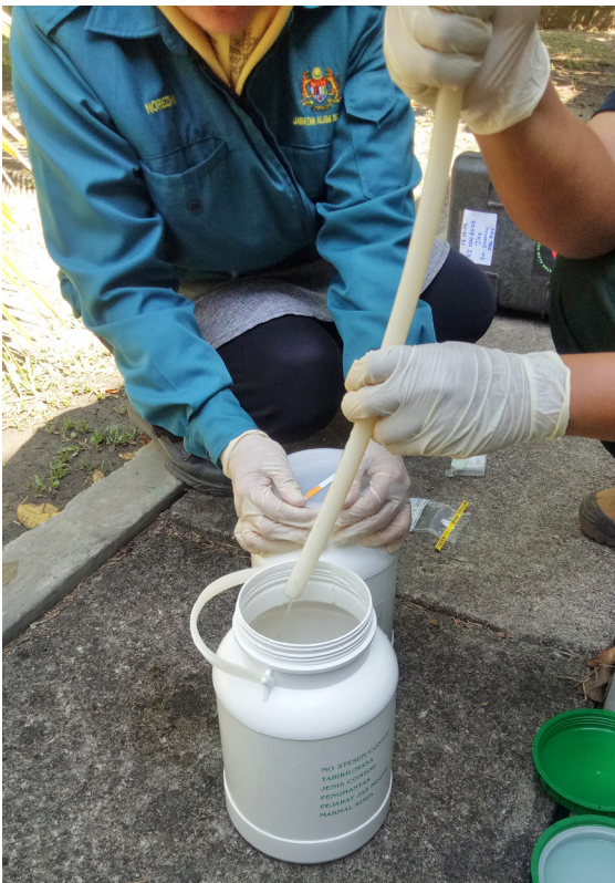
Kerja-kerja Persampelan Air Tanah Mengikut SOP Program Pengawasan Kualiti Air Tanah Sampling Process of Groundwater According to SOP of Groundwater Quality Monitoring Programme
