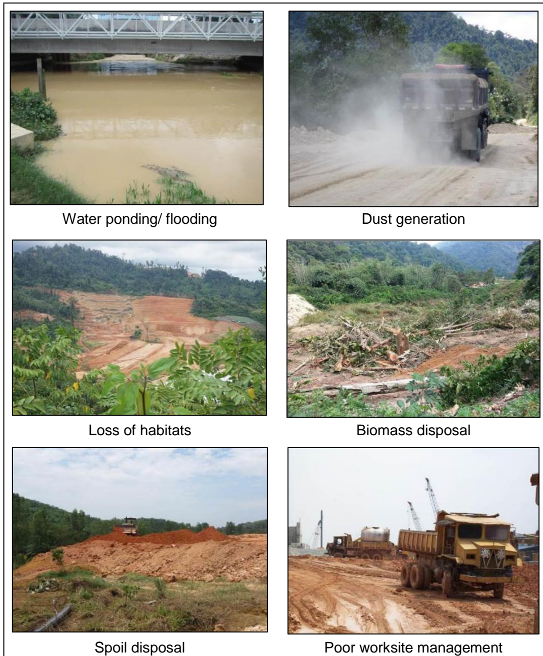
Figure 5.3 (b): Photo Inventory of Common Impacts Associated with Iron and Steel Industry
