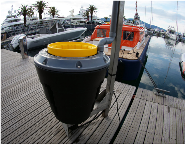
Seabin before its installation
