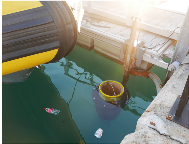
Sea bin in the water after installation
