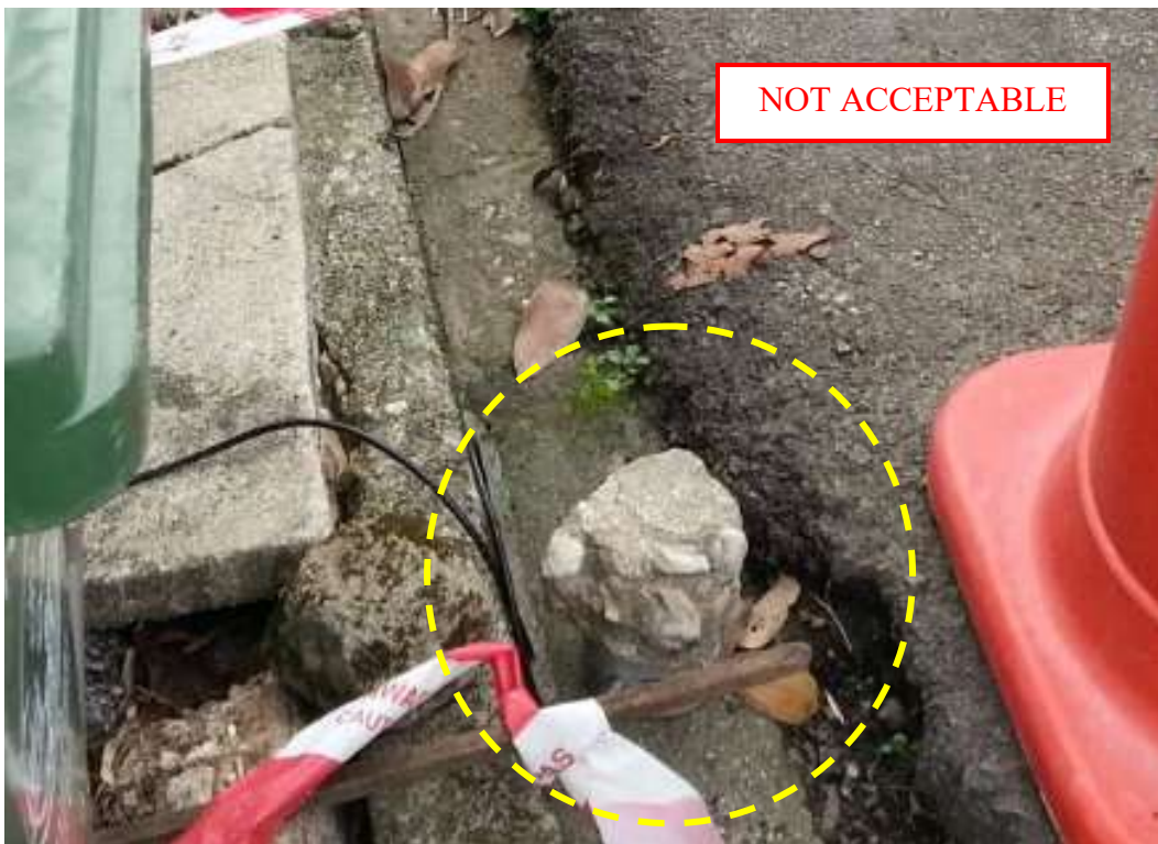
Plate B-24: Geophone sensor placed onto solid ground held in place with small rock. Sensor should instead be stud fastened onto base plate and epoxy bonded onto ground
