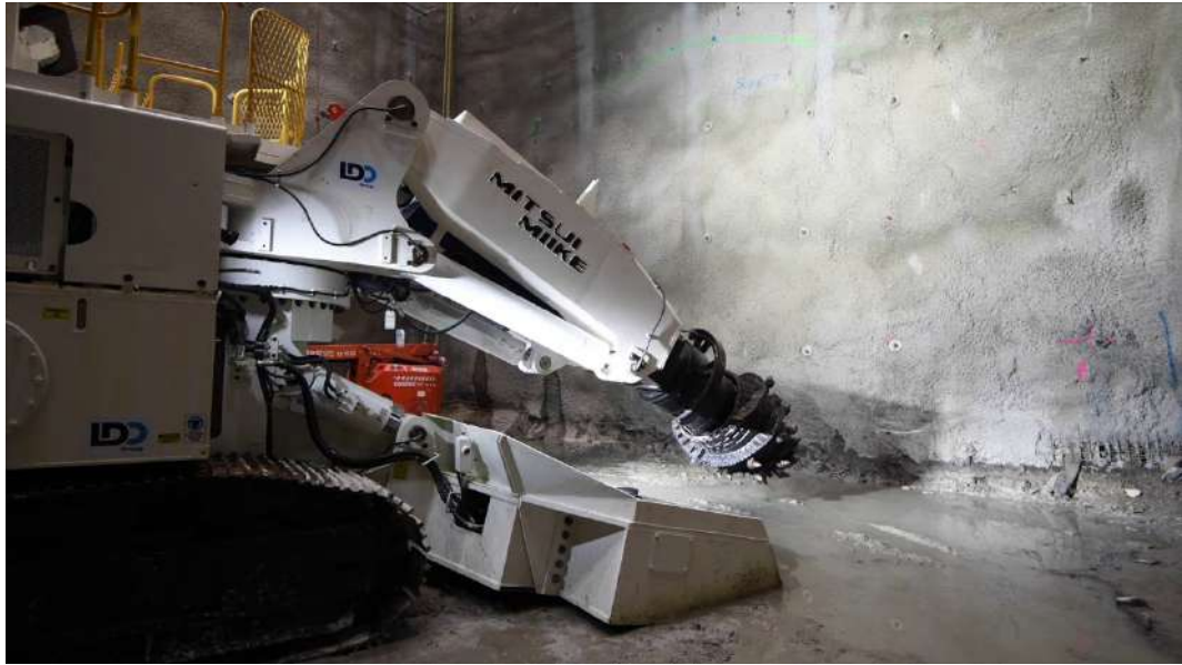
Plate E-17: Road-header used in underground railway tunnelling works (Cross River Rail, Australia)
