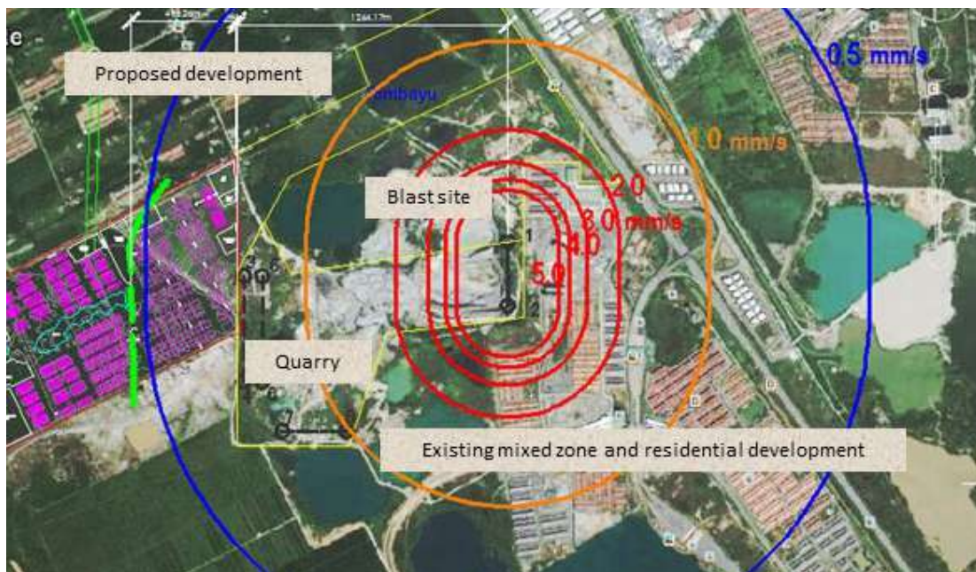
Plate 11-1: Vibration map showing predicted ground vibration contours from blasting site.
