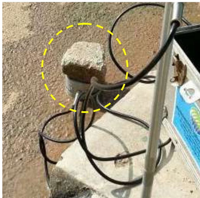
Plate B-22: Geophone sensor placed onto solid ground held in place with small rock.
