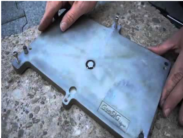
Plate B-11: Mounting plate (OEM accessory) for vibration monitoring system being bolted onto building structure for rigid coupling of equipment (built-in sensor) to building foundation
