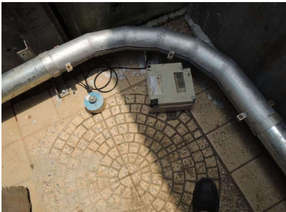
Plate B-4: Vibration monitoring unit with accelerometer sensor for measurement at work site
