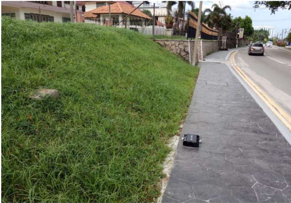
Plate B-6: Vibration monitoring unit (integrated sensor type) used for baseline measurement at residential location.
