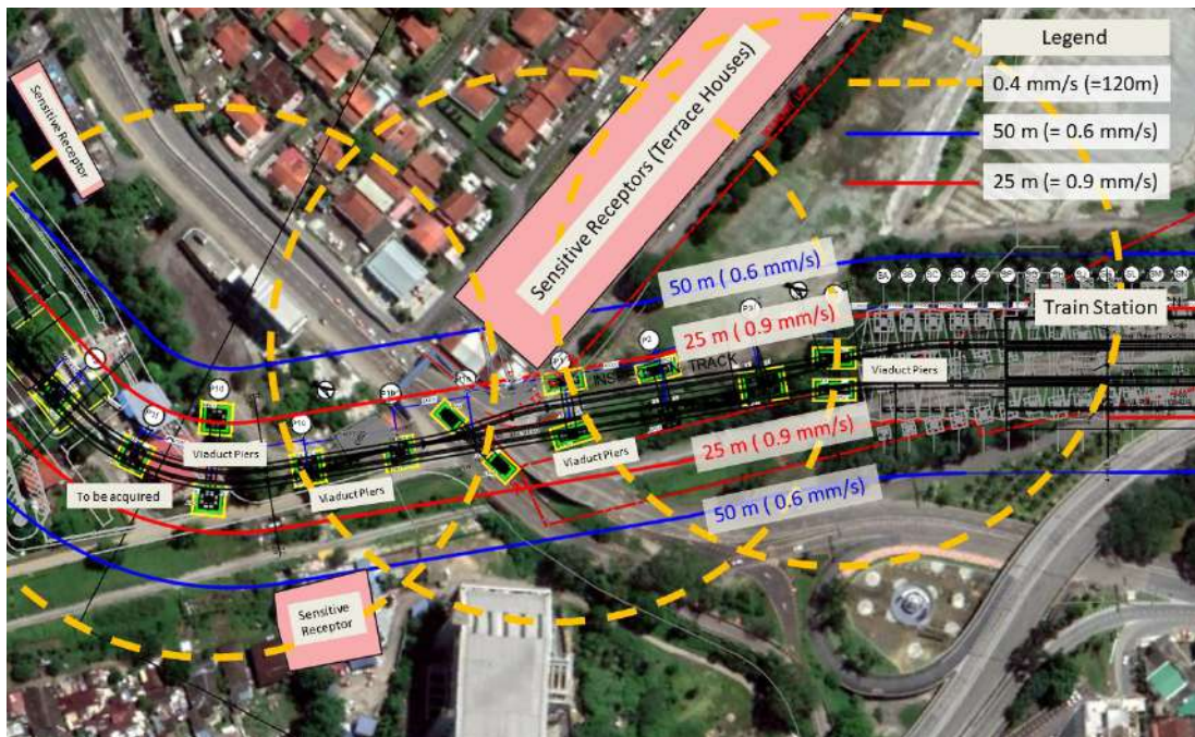
Plate 11-2: Vibration map showing predicted ground vibration zone of influence from piling locations for different critical distances and corresponding levels.
