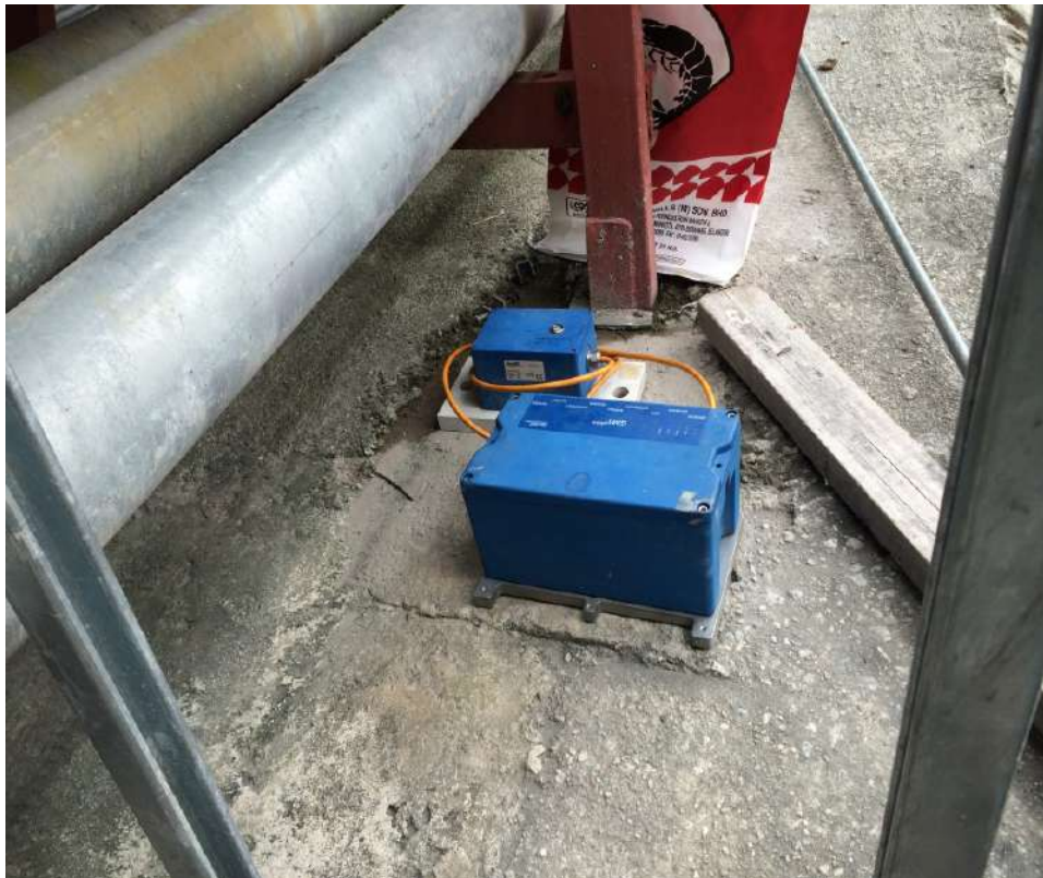
Plate B-4: Vibration monitoring unit with accelerometer sensor for measurement at work site
