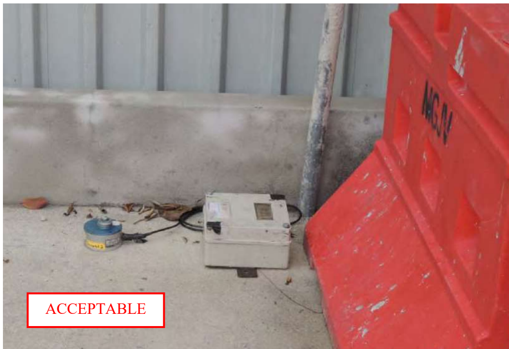
Plate B-17: Geophone sensor bolted directly onto hard surface (without using a mounting plate with spikes).
