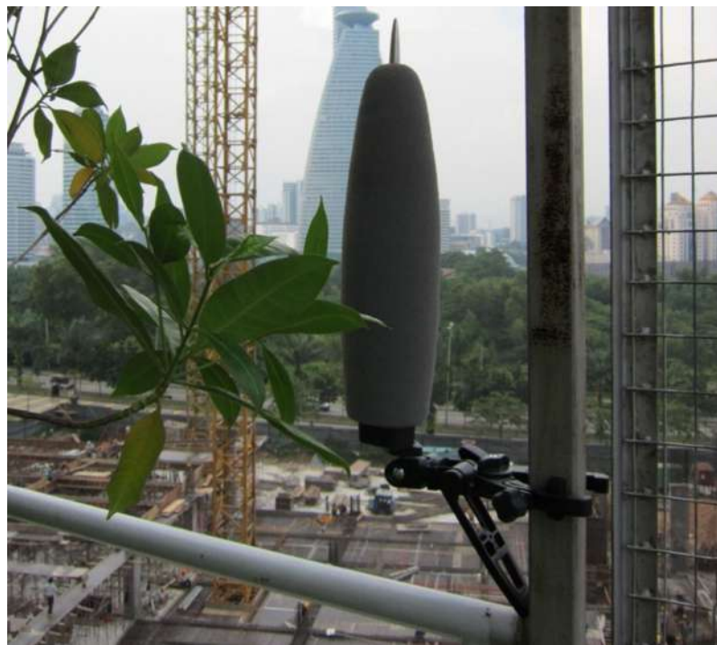
Figure B-2: Example of semi-permanent and permanent outdoor monitoring unit
