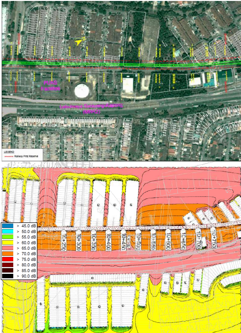
Figure 7: Noise contours ( L_{\max} levels) on grade for transit trains from 3D noise modelling of trains pass by on elevated viaducts to the environment
