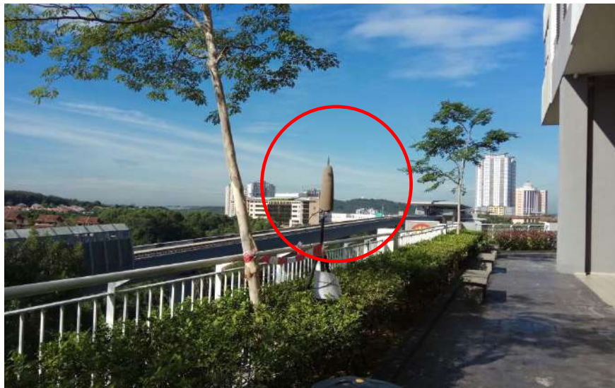
Figure B-13: Example of noise measurement at open terrace in a high-rise building
