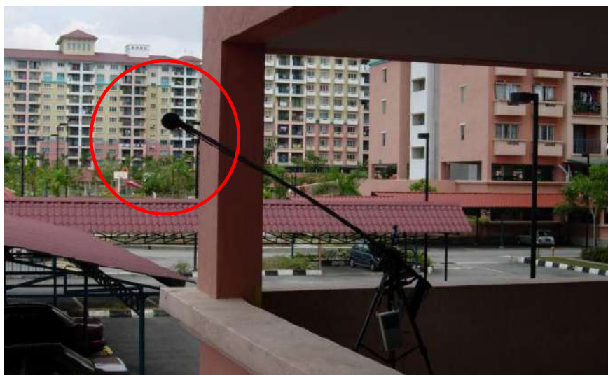
Figure B-14: Example of microphone located beyond building facade
