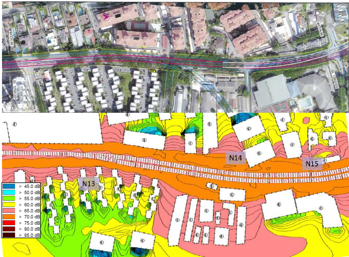
Figure 4: Noise map ( L_{10} levels) of a proposed elevated highway to be built amongst existing developed area
