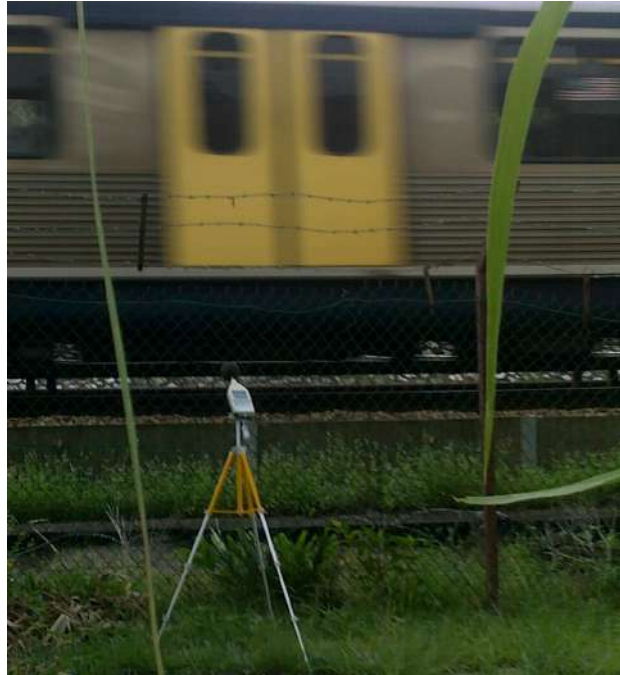
Figure B-11: Example of noise measurement of trains pass by noise on grade
