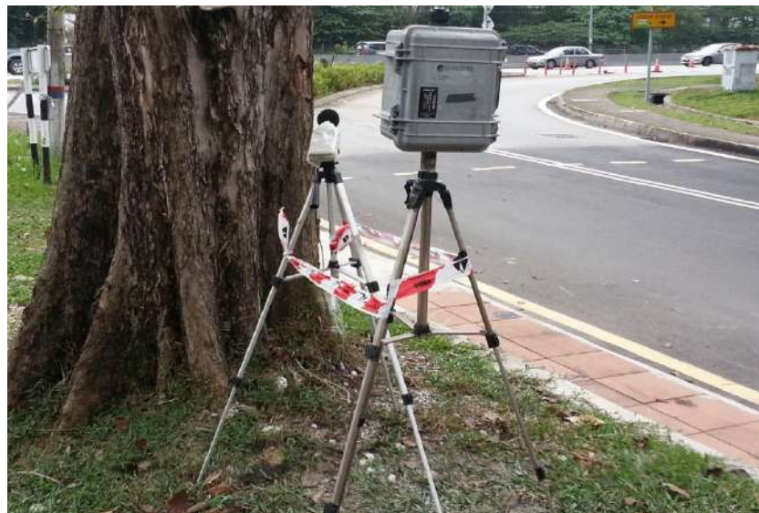
Figure B-17: Example of unacceptable monitoring in progress with sound level meter obstructed by objects (and adjacent extraneous noise source)
