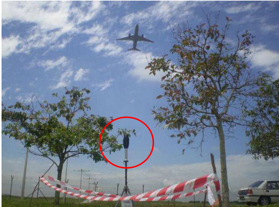
Figure B-38: Example of microphone position in aircraft noise measurements
