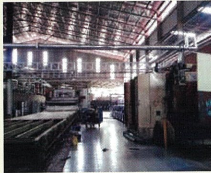
A transparent wall allows daylight into the factory and avoid the use of electric powered lamps during the day.
