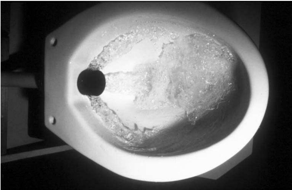
Figure 11.3 WC bowl design for a 4 litre flush volume as used in the Gaberone project (Courtesy of Heriot-Watt University)
