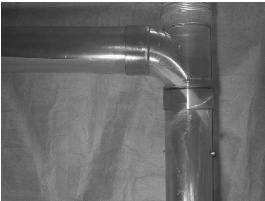
Figure 4.14 Discharge from a WC branch entering a vertical stack, illustrating the formation of annular flow. The internal view illustrates the reduction in air path cross section below the active junction (Courtesy of Heriot-Watt University)
