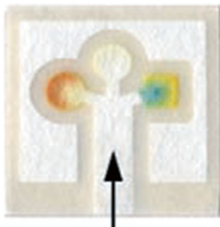
Fig. 12.2 Patterning hydrophobic barriers using wax printing. (a) Devices are prepared using inexpensive equipment: device layouts are designed using computer software (1), a commercially available printer prints solid wax ink onto paper (2), and a hot plate or other heat source reflows the wax to create hydrophobic channels throughout the thickness of the paper (3). (b) Demonstration of a three-channel device advanced from concept to working prototype. (c) Cross-sectional schematic illustration of a device before and after heating to reflow printed wax. Adapted with permission from Carrilho et al. [60]. Copyright 2009 American Chemical Society
