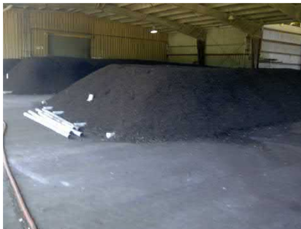
FIG. 29.7 A forced air compost pile used to treat vegetative, food, and animal wastes.
