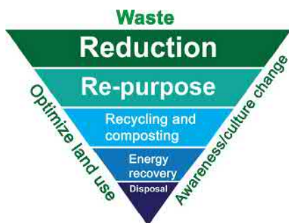
FIG. 29.1 The Net Zero Waste Hierarchy Diagram.
