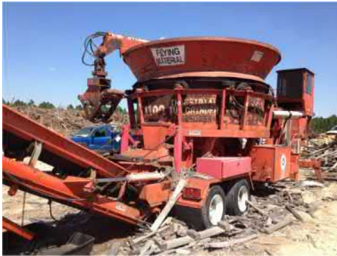
FIG. 29.6 Tub grinder, an effective tool to reduce volume of large debris materials, including chipping of woody vegetative material.
