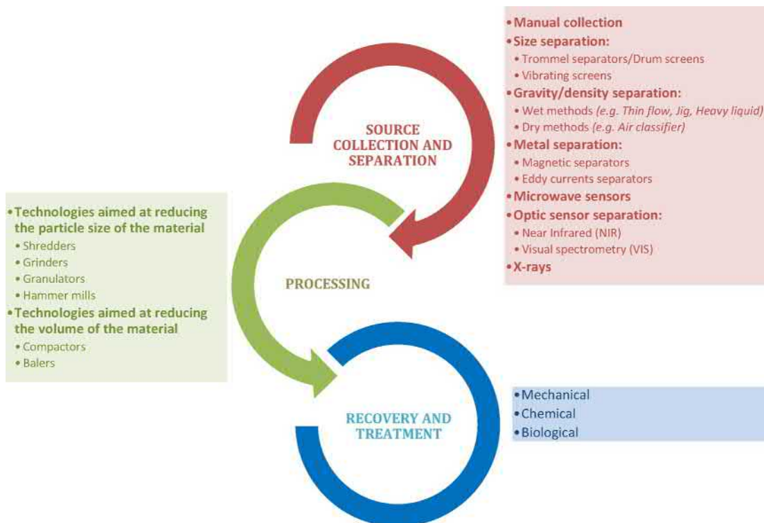
FIG. 19.5 CW recycling and recovery technologies.
