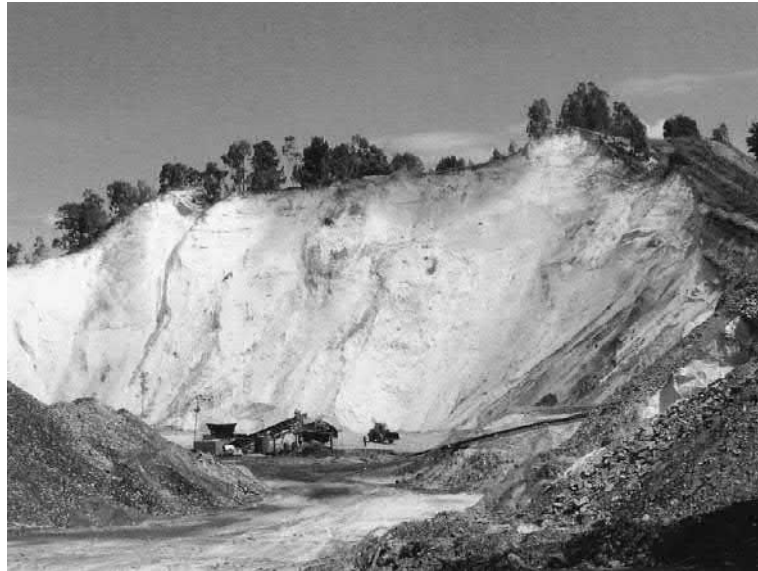
FIG. 6.1 A 100-year-old dump of gold tailings sand being remined for processing to extract the uranium and residual gold content.
