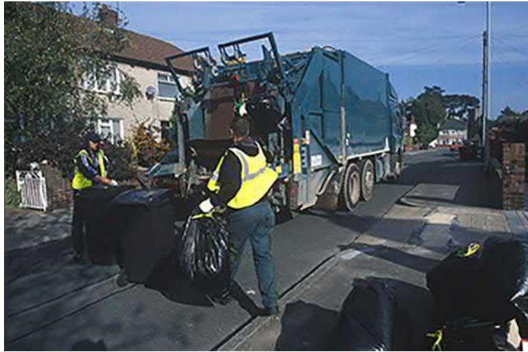
FIG. 4.4 Rear-loading refuse collection vehicle. From https://partners.wrap.org.uk/assets/7471/ . Used with permission from WRAP.
