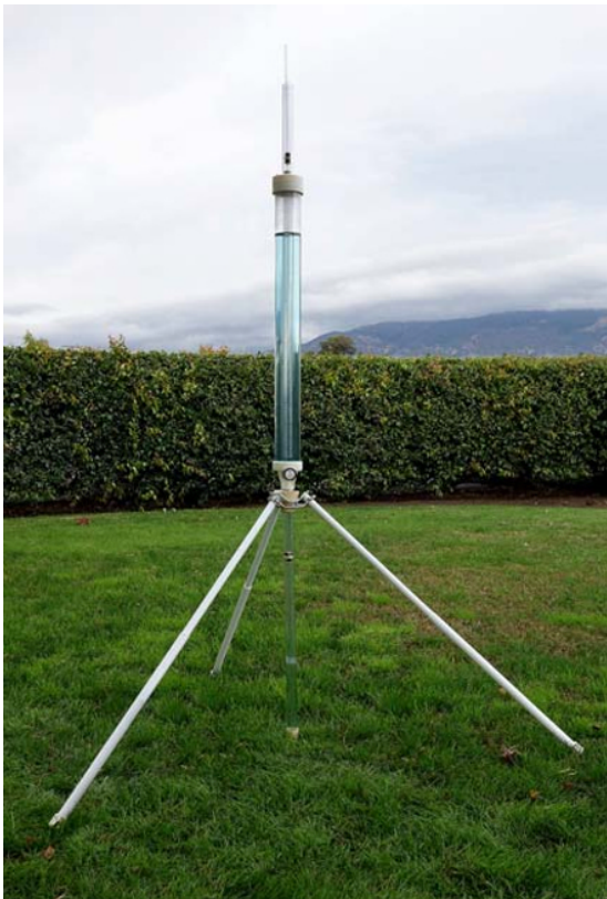
Fig. 18.3 Guelph Permeameter. Photograph reproduced with permission from Soilmoisture Equipment Corporation. (See insert for colour representation of the figure.)
