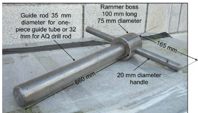
Fig. 7.13 Rammer for hammering guide tube into the soil.
