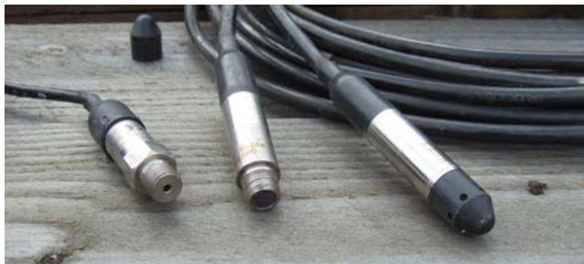
Fig. 12.11 Pressure transducers. The one on the left has a pressure port, while the other two are flush diaphragm transducers. The one on the right has a protective cap over the diaphragm for water level monitoring applications.
