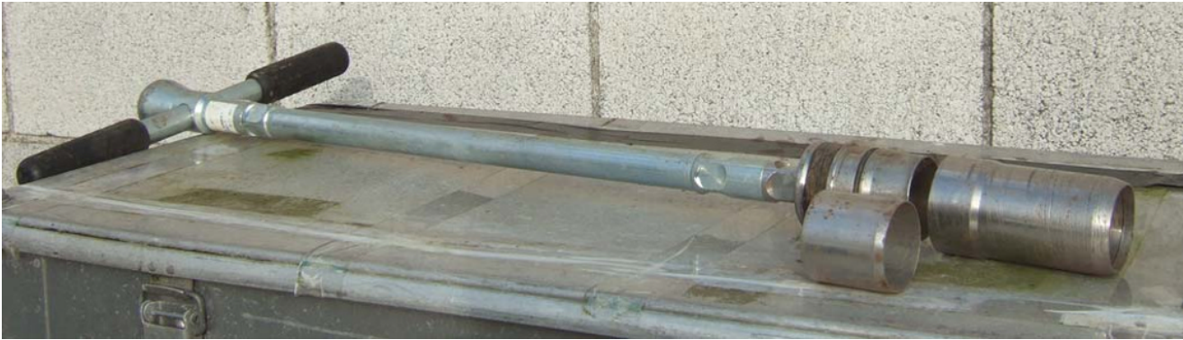
Fig. 6.2 Soil sampler showing sharpened body, removable retaining sleeve and shaft to allow sampling at depth. This one does not have a sliding hammer. Instead, the handle is used to hold it steady, while the sampler can be driven into the soil by blows to the heavy boss at the top.
