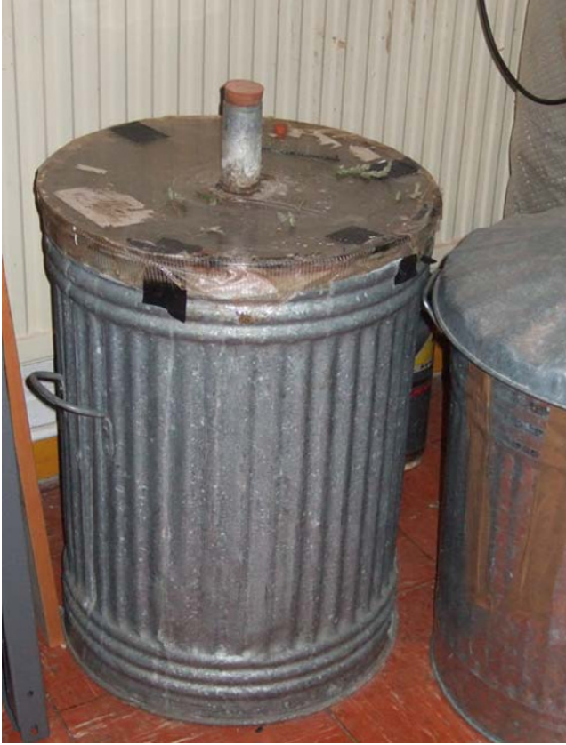
Fig. 7.22 Water drum. The transparent cover allows the water level and clarity to be monitored. To prevent growth of algae, the drum should be covered with an opaque lid when not in use.
