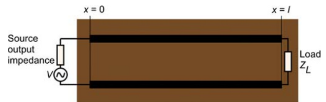
Fig. 8.17 Transmission line terminated with a load, Z_L .
