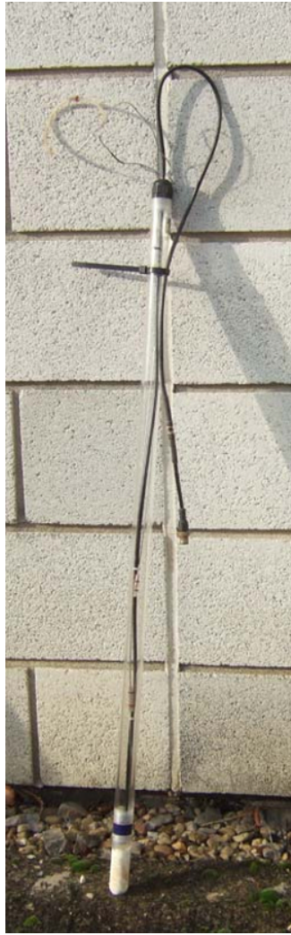
Fig. 12.10 UMS T4e tensiometer showing the filling tubes connected by a flexible plastic tube at the top.
