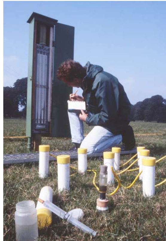
Fig. 12.20 A set of mercury manometer tensiometers showing scale, radiation shielding, syringe and water supply for purging. Reproduced with permission of the Centre for Ecology & Hydrology.
