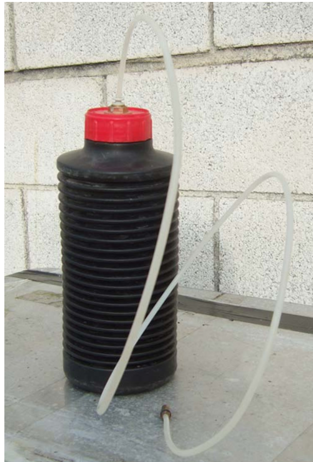
Fig. 12.36 Collapsible plastic container for storing de-aired water. A check valve is attached to the end of the plastic tube to prevent air from being sucked into the bottle.
