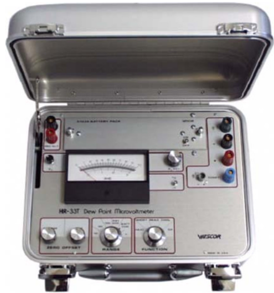
Fig. 14.2 The Wescor HR-33T manual psychrometer reader. Reproduced with permission of Wescor Inc., Logan Utah.
