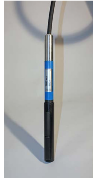
Fig. 8.27 IMKO Trime IPH depth probe showing the four spring-loaded plates on one side to ensure good contact with the inside of the access tube. Photograph reproduced with permission of IMKO GmbH.
