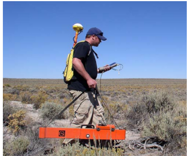
Fig. 21.6 Geonics EM38-MK2 in use in the field. The instrument is carried close to the ground surface and the operator has a portable GPS system on his back. Both instruments are connected to a handheld field data logger. Photograph reproduced with permission from Geonics Ltd.
