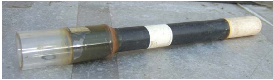
Fig. 12.14 Tensiometer with separate air trap bonded to the body tube with epoxy.
