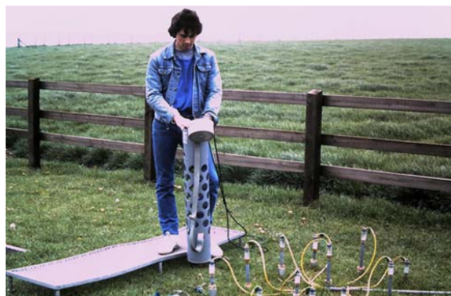
Fig. 7.5 A neutron probe in use in the field. © NERC (CEH). Reproduced with permission.
