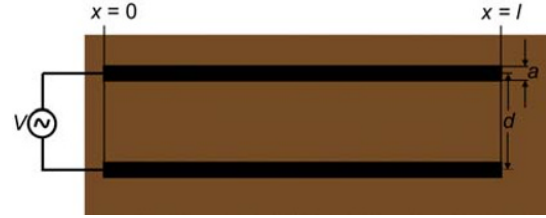
Fig. 8.14 Schematic transmission line embedded in a medium, connected to an alternating voltage source, V .
