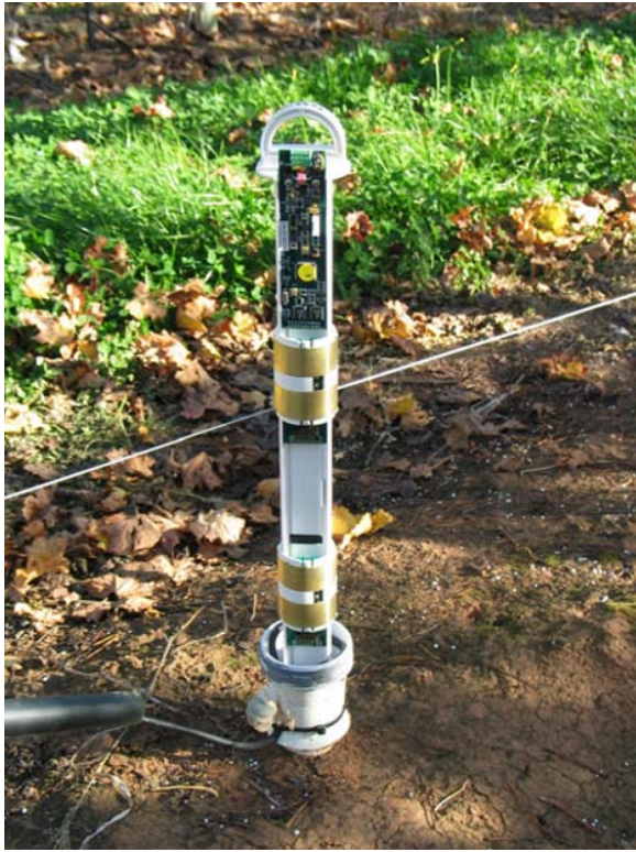
Fig. 8.39 Sentek EnviroScan capacitance probe system showing the two cylindrical electrodes of each sensor unit. The printed circuit board of each unit is located inside the rings, with the main control board at the top. The ribbon cable connecting each sensor's printed circuit board to the main control board runs behind the plastic partition between the sensors. In operation, the complete assembly is placed inside the plastic access tube, the top of which can be seen protruding above the ground surface. Photograph reproduced with permission of Sentek Pty, Australia. (See insert for colour representation of the figure. )
