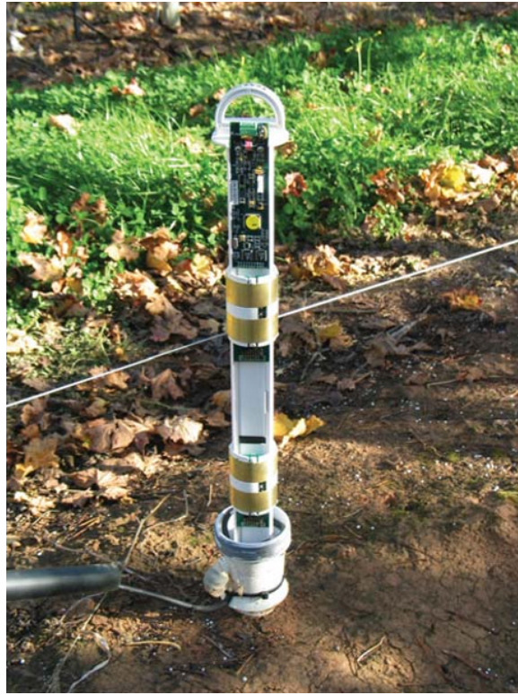
Fig. 8.39 Sentek EnviroScan capacitance probe system showing the two cylindrical electrodes of each sensor unit. The printed circuit board of each unit is located inside the rings, with the main control board at the top. The ribbon cable connecting each sensor's printed circuit board to the main control board runs behind the plastic partition between the sensors. In operation, the complete assembly is placed inside the plastic access tube, the top of which can be seen protruding above the ground surface. Photograph reproduced with permission of Sentek Pty, Australia.
