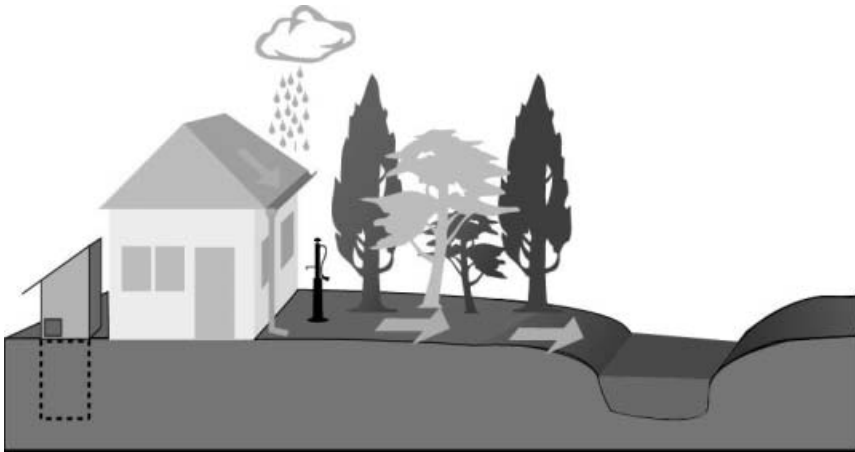
Figure 22.9 Filter strip and swale in an urban landscape. (Adopted from UNEP, 2002).
