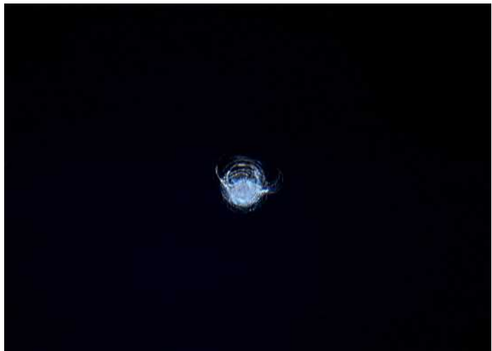
FIG. 30.1 Damage to the Cupola window of the International Space Station, about 7mm across; probably due to a paint flake impact (© ESA/NASA).
