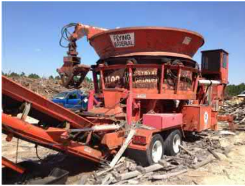
FIG. 29.6 Tub grinder, an effective tool to reduce volume of large debris materials, including chipping of woody vegetative material.
